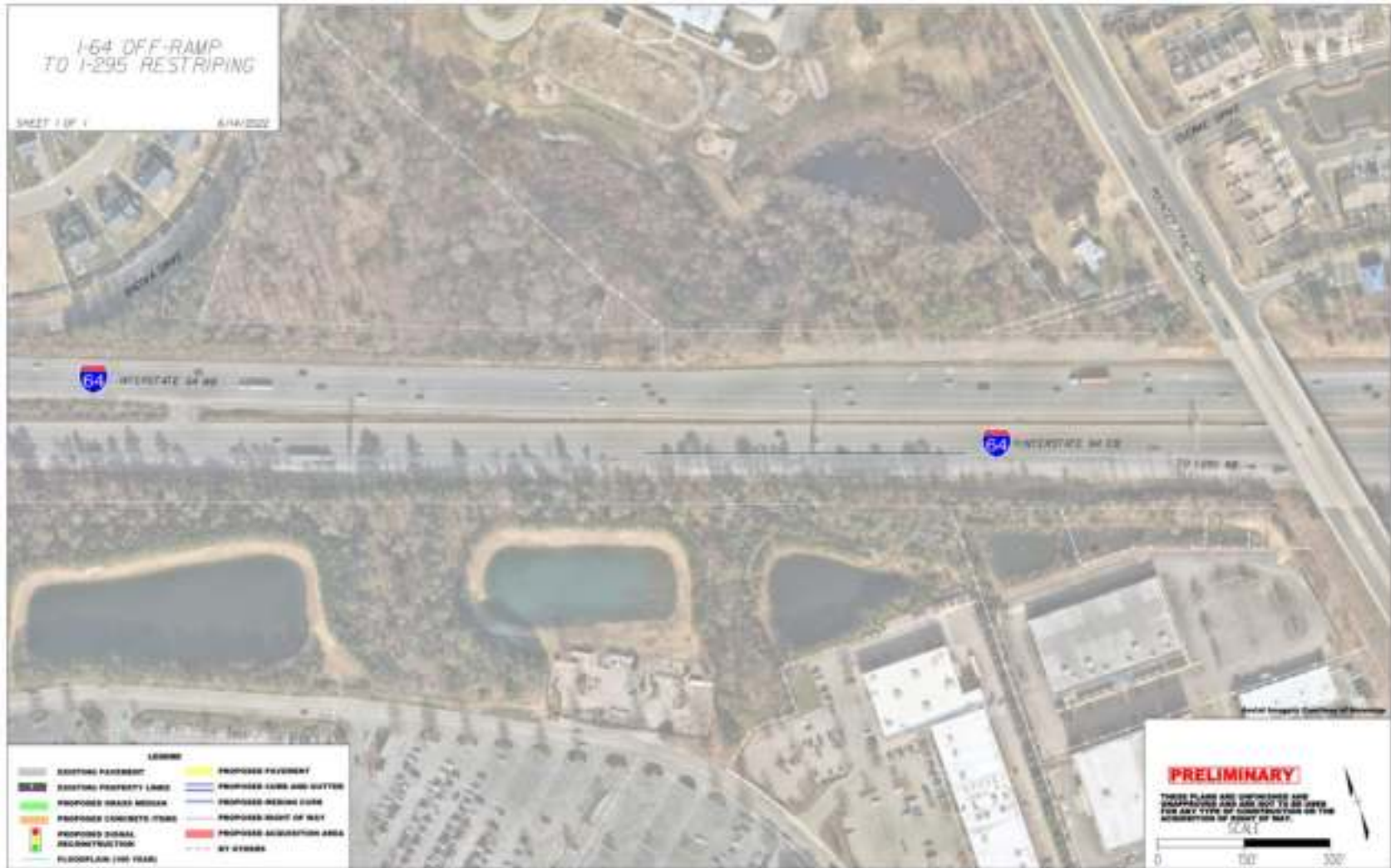
Figure 38: I-64 to I-295 Diverge Reconfiguration
