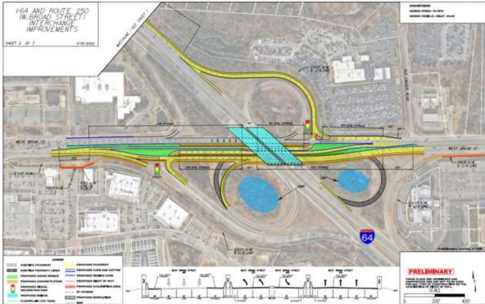
Figure 29: US 250 at I-64 Partial Cloverleaf Improvement (2)
