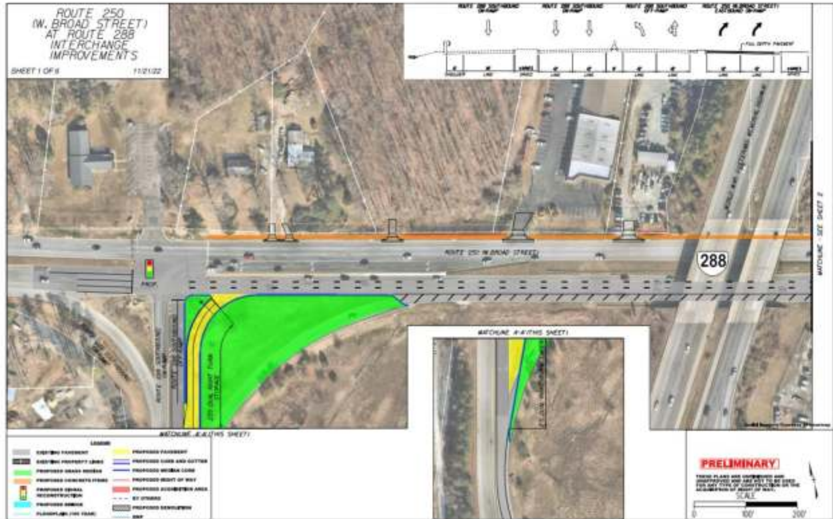
Figure 31: Route 288 at US 250 Ramp and Ramp Terminal Improvements (1)
