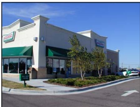
The location of windows and landscape design allow customers and employees to see into and out of this business. This is a form of Natural Surveillance .
