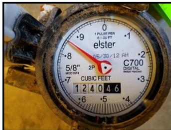
The white triangle in the middle of the meter is the leak detector. If the triangle is rotating while water is flowing through the meter.
