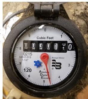
The blue circle is the leak detector. If the blue circle is rotating while water is flowing through the meter.
