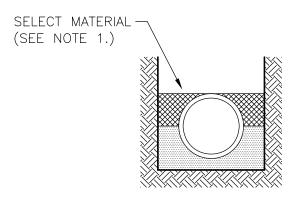
PIPE BEDDED TO ITS CENTERLINE IN COMPACTED GRANULAR (SEE NOTE 2) MATERIAL, 4" MINIMUM UNDER PIPE. COMPACTED GRANULAR OR SELECT MATTERIAL<sup>3</sup> TO TOP OF PIPE. (APPROXIMATELY 90% STANDARD PROCTOR, AASHTO T-99.)
