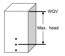
The maximum head acting on the perforations is the difference in elevation between the water quality volume elevation and the midpoint between the upper and lower perforation elevations. If there is only one perforation, that elevation will be the midpoint elevation.
