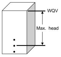
The maximum head acting on the perforations is the difference in elevation between the water quality volume elevation and the midpoint between the upper and lower perforation elevations. If there is only one perforation, that elevation will be the midpoint elevation.
