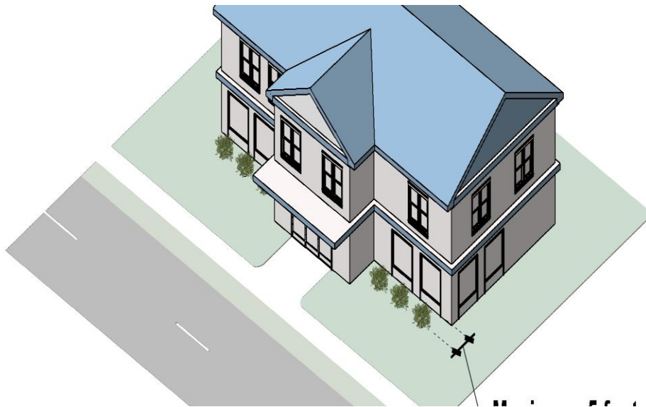
Figure 5309A: Foundation Planting Requirements
